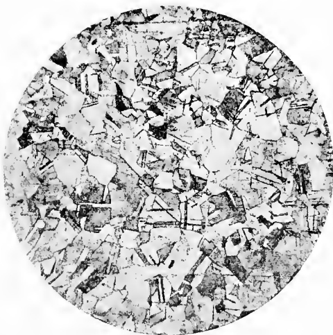
B. Brass (Cu 70, Zn 30%) annealed. \times 86 .
